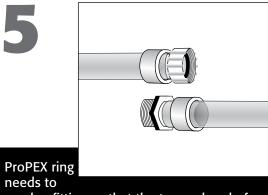
overlap fitting so that the tapered end of the fitting is visible beyond the ring.
